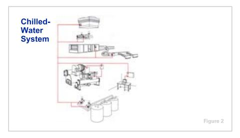
Water chillers are used in a variety of air conditioning and process cooling applications. They are used to make cold water that can be transported throughout a facility using pumps and pipes. This cold water can be passed through the tubes of coils to cool the air in an air conditioning application, or it can provide cooling for a manufacturing or industrial process.
